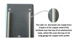
When the measurement is taken between the tester's two mesh rails, the tester will indicate the surface resistivity of the material being tested.
