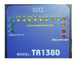
The test value is indicated on the LED display. Half decades provide greater accuracy by giving closer indication to the measurement value. A decade will brighten to the according test result. LED colors signify the test values.
