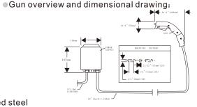
compressed air must be clean, dry and oil free. The maximum allowable input pressure is no more than 100 PSI(7bar). We suggest using external pressure regulator and filter / dryer. Line voltage is supplied to the power unit must measure up with related standard and have good grounding. Do not ignore equipping the grounding line.
